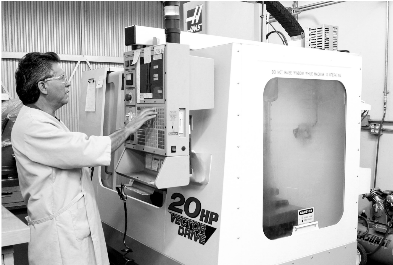
Juan Alvarez, CNC Machinist sets up Milo Engineering's Haas VF0 milling machine retrofitted with a Renishaw MP10 probe system.
