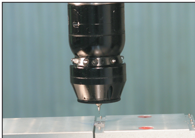
Close up of Renishaw MP-10 probe checking dimensions on the small Kovar subplate produced at Milo Engineering for Northrup Grumman.
